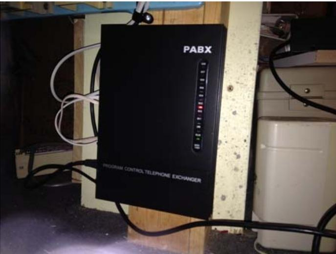
The new PABX phone system has eight internal lines and one external connection. The NCL does not use the external connection and currently only uses three internal connections for the dispatcher, hostler and yardmaster.
