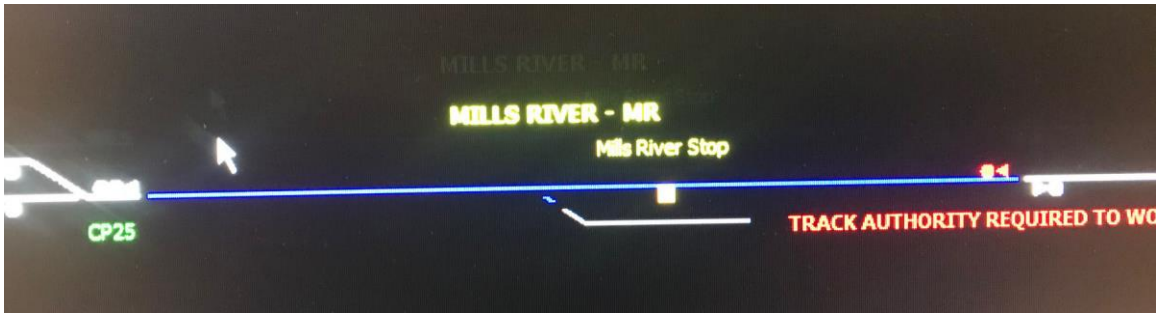
Track Authority has been granted to the above block which changes color to Blue. Signals on either end of the block indicate 'Stop'.
