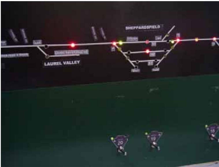
amber LEDs designate turnout positions. On the mainline, green indicates the turnout is in the normal position, amber indicates the turnout is in the reversed position. In staging areas, all turnout positions are indicated by amber LEDs that show train routes in each staging yard. The Dispatcher controls mainline turnouts by pushing momentary toggle switches on the console for the corresponding turnout.
